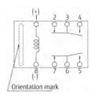
PC board mounting hole layout (BOTTOM VIEW)
