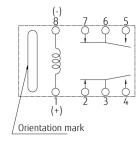
PC board mounting pad layout (TOP VIEW)
