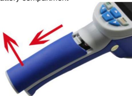
2. Remove the old batteries and install new batteries.
