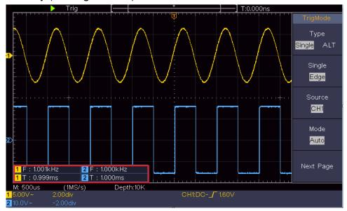
Figure 4-13 Automatic measurement
