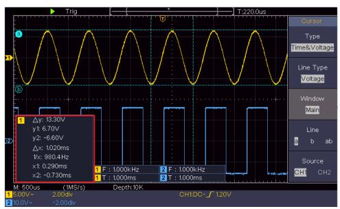
Figure 4-16 Time&Voltage Cursor Measurement
