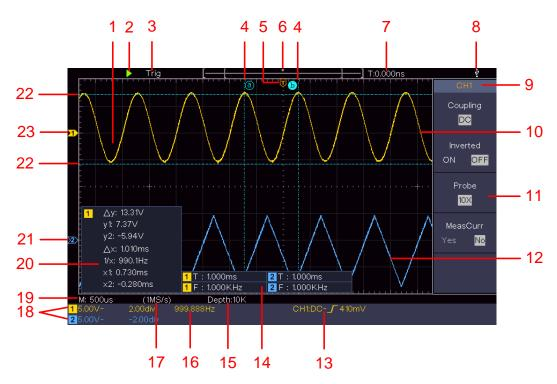
Figure 3-4 Illustrative Drawing of Display Interfaces
