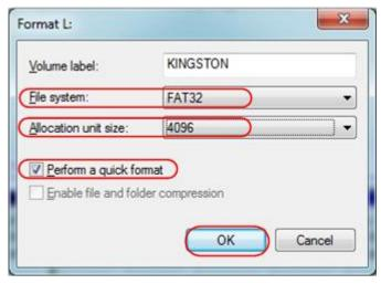
Figure 4-4: Formatting the USB disk setting
