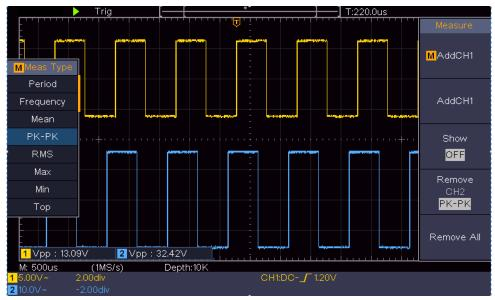
Figure 6-2 Waveform of Gain Measurement
