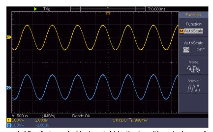
Figure 4-12: Autoscale Horizontal-Vertical multi-period waveforms
