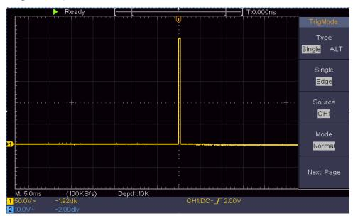
Figure 6-3 Capturing a Single Signal
