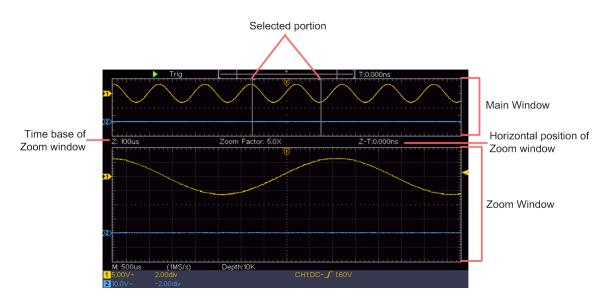
In normal mode, the **Horizontal Position** and **Horizontal Scale** knobs are used to adjust the horizontal position and time base of the Main window. In wave zoom mode, the **Horizontal Position** and **Horizontal Scale** knobs are used to adjust the horizontal position and time base of the Zoom window.
