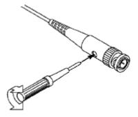
Figure 3-7 Adjust Probe
