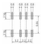
PC board mounting pad layout (TOP VIEW)
