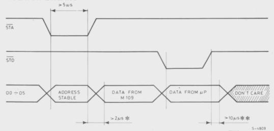
\* The data from the M109 can be read after a time  $> 2 \mu s$  from the positive going edge of  $\overline{STA}$ .
